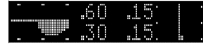
2 seconds later, the car is braking at .30 G. The peak braking G-Force over the past 4 seconds is .60 G. The car is beginning a right turn, cornering at .15 G.
