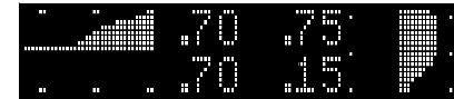
2 seconds later, the car continues to accelerate, and is now cornering at .15 G.
