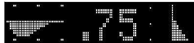
2 seconds later, the car is no longer braking, but it is cornering to the right at .75 G. (The peak G-Force over the past 4 seconds is .75 G.)
