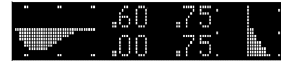
2 seconds later, the car is not braking, but the peak braking G-Force over the past 4 seconds is .60 G. The car is cornering to the right at .75 G.
