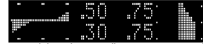
2 seconds later, the car is still cornering at .75 G, and is accelerating at .30 G. The peak accelerating/braking G-Force over the past 4 seconds is .50 G.
